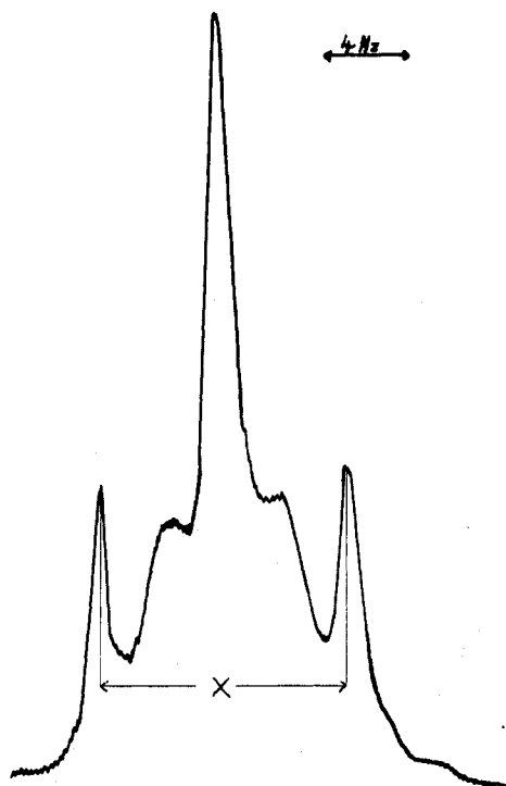
Figure 2. Proton nmr spectrum (methyl protons) for complex cations [\text{IrL}_4]^+ [ \text{L} = \text{P}(\text{OMe})_2\text{Ph}, \text{P}(\text{OMe})\text{Ph}_2 ].
